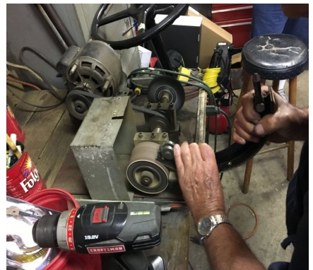
“Arcing” shoe to fit the drum.
