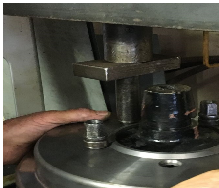
Pulling drum and hub together, needs to be tight.
