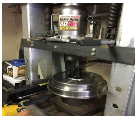
Pulling drum and hub together, needs to be tight.
