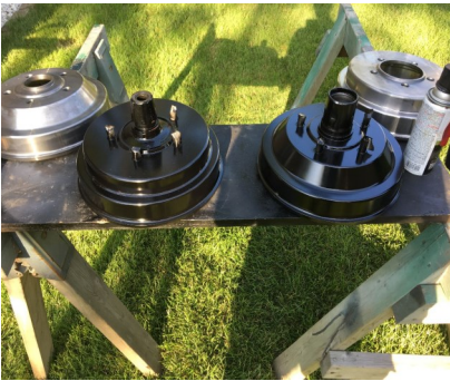
Drums, before and after paint.
