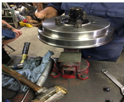
Pulling drum and hub together, needs to be tight.
