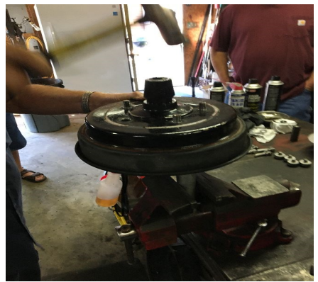
Drilling out studs with 5/8" hole and pounding them out to reuse the hubs.
