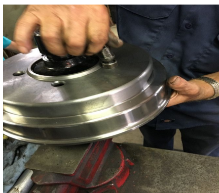
Pulling drum and hub together, needs to be tight.
