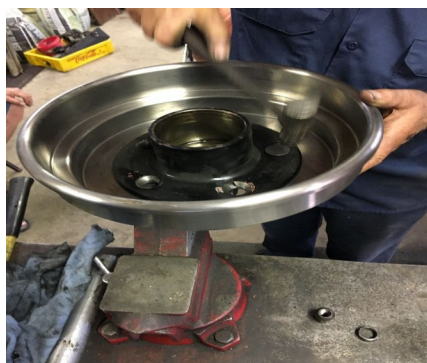
Pounding in new studs.
